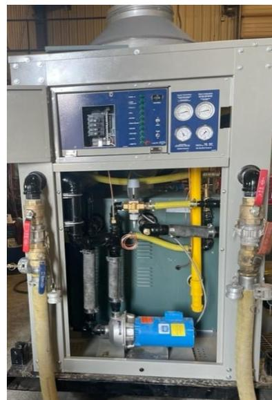
Figure 28 - Primary Circulation Line Connections
