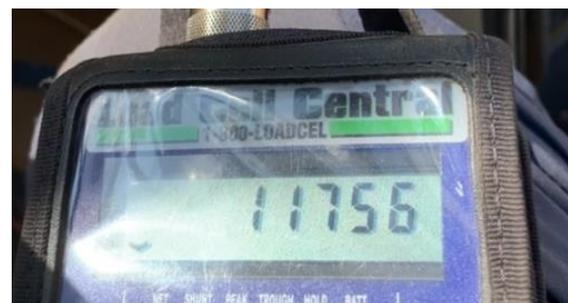
**Figure 4.** Peak force applied during the lifting frame test.
